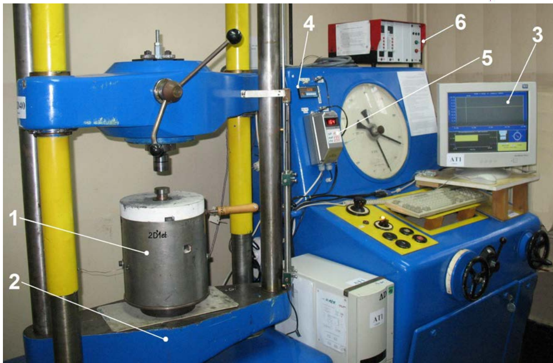
ECAP rig for 8 mm×8 mm billets (classical channel 1×90°, metal forming type: shearing): 1--ECAP tool (2D'1et), 2--400 kN hydraulic press, 3--DAQ computer system, 4--force measurement system, 5--stroke measurement system, 6--temperature controller
